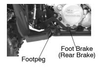
**WARNING!** Aggressively applying the foot brake when backing down a hill may cause rear tipover, which could result in serious injury or death. Never back down a hill. Use caution when applying the foot brake. Do not aggressively apply the foot brake when going forward. The rear wheels may skid and slide sideways, causing loss of control.
